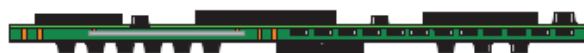
Mother board with embedded die and passive components. SMA components on top.
